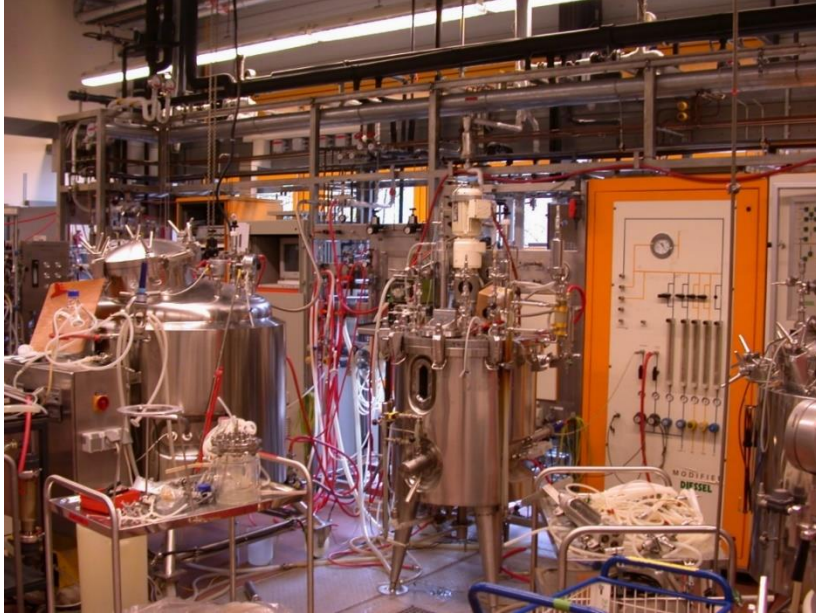
1990: GBF's 100 l Pilot Plant for cell culture-based bioprocess research
