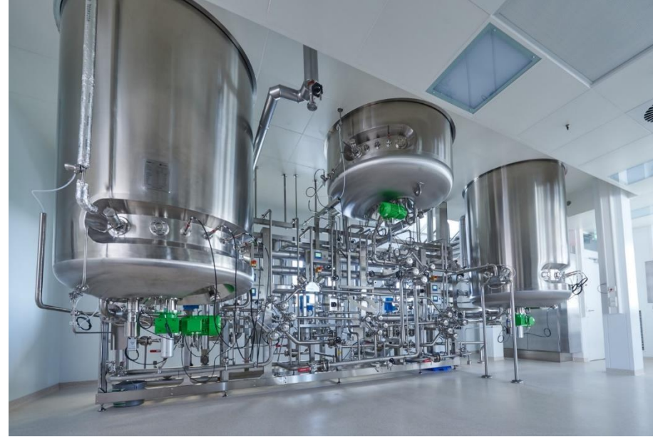
2015: Rentschler's 2x 3000 l TWIN Facility for cell culture-based biopharmaceutical manufacturing
